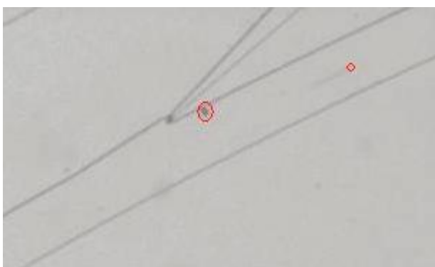
Figure 23: Still image from a video depicting polystyrene beads flowing past a filled pocket without entering the pocket. This demonstrates single trapping.
